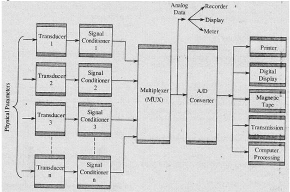
fig.9.b. Generalised Data Acquistion System
