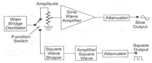
fig.6.a.(ii) AF sine & Square wave generator
