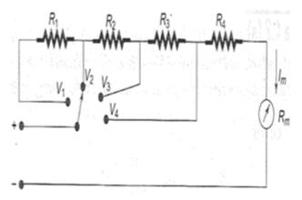
fig 4.a.(ii) Multiplier Connected in Series String
