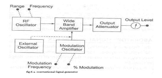
The carrier frequency is generated by a very stable RF oscillator using an LC tank circuit, having a constant output over any frequency range. The frequency of oscillations is indicated by the frequency range control and the venire dial setting. AM is provided by an internal sine wave generator or from an external source.
