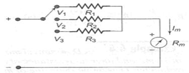
fig.4.a.(iii) Multirange Voltmeter
