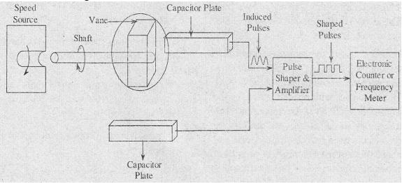
fig.8.b. Capacitive Transducer
