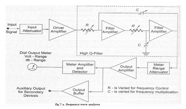
The complex wave to be analyzed is passed through an adjustable attenuator, which serves as a range multiplier and permits a large range of signal amplitudes to be analyzed without loading the amplifier
